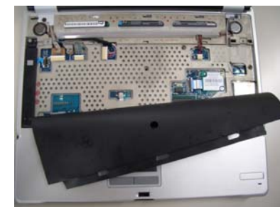
Spill-resistant Keyboard - A layer of bending insulation beneath the keyboard holder to cover areas that would otherwise be exposed.
