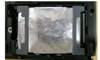
Shock absorber material is added around the hard drive disk and works as a corner bumper mechanism
